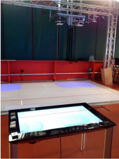
Figure 1: Hardware setup consisting of SUR40 tangible tabletop display and augmented floor surface
