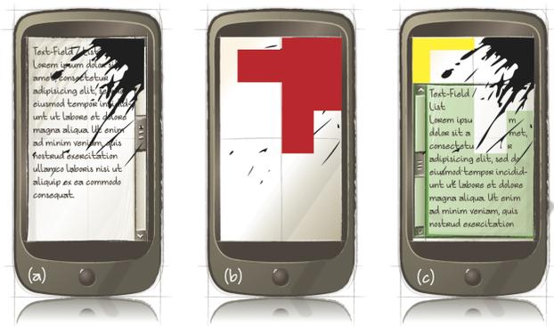
**Figure 10. Adaptive content rendering example:** (a) A text area is partially occluded by display damage. (b) The user marks the damaged area on a grid (red). (c) An adaptive text renderer floats the text around the damaged area (green) and moves the scroll indicator to the left. In this scenario, the upper-left corner can also not be used anymore (yellow).
