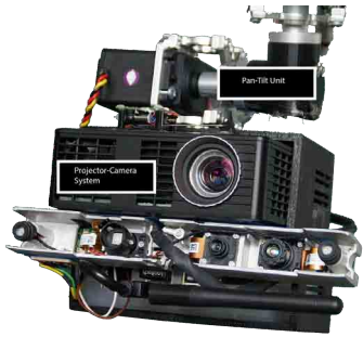
Figure 1: The UbiBeam System a Compact and Steerable Projector-Camera System
