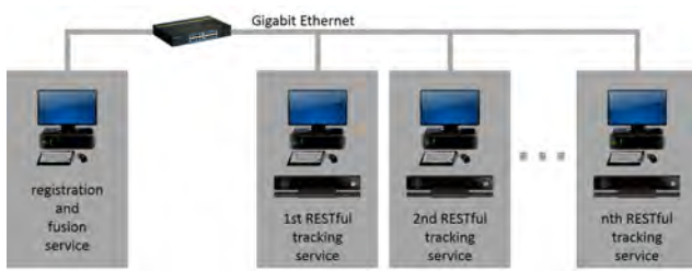
Figure 9: Hardware setup for the tracking system with service-oriented, distributed sensor services
