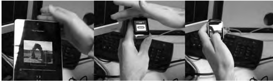
Figure 12.8: Display Copy system example: After the smartphone is touched long with the ring it displays a clipping frame to select the start view for a connected smart watch and finally stores a copy of the display and the selected region (left). Touching the smart watch with the ring for a short time is recognized (middle) and shortly afterwards the picture is retrieved from the server (phone) and can then possibly be panned and zoomed on the watch (right).
