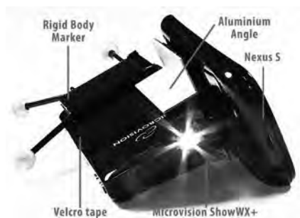
Figure 8.14: The IPC hardware prototype. A SHOWWX+ Pico Projector is equipped with retro reflective markers and by two aluminum angles and Velcro tape orthogonally and with height offset (for better handling and larger projection) attached to a Nexus S phone.
