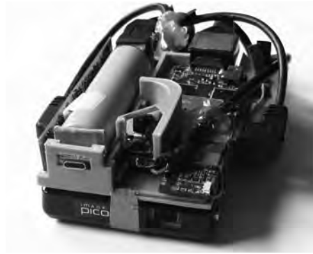
Figure 10.5: The interior design of the SpiderLight system showing the projector at the bottom, the Android TV stick with the camera mirror on the right, and the battery on the left side. Not visible is the x-IMU which sits behind the projector on the lower side.
