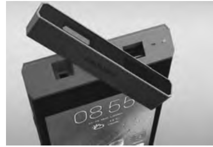
(b) The Lenovo Smart Cast concept. A rotatable mirror at the top allows to flip the direction between forward and backward of camera and projector at once (does not allow arbitrary rotations, though). Image courtesy of Lenovo.
