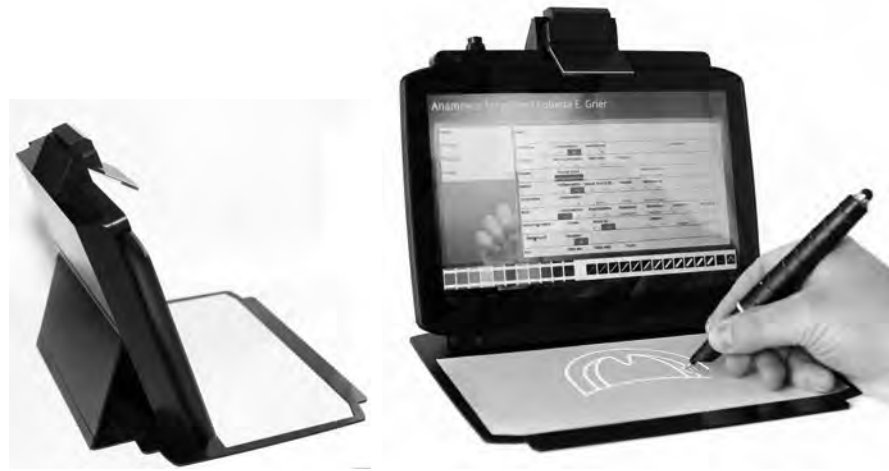
Figure 6.1: The Penbook setup: a tablet computer with an integrated projector augments a paper on its lid, transforming it to a display that supports digital hand-writing with light instead of ink.
