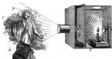
(a) Inner workings of a magic lantern
