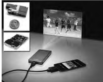
Figure 2.5: The Microvision SHOWWX accessory series (SHOWWX 10 Lumens shown) using Microvision's PicoP engine (top left). The SHOWWX+ HDMI (15 Lumens) was used in all projects presented in this thesis except for the AMP-D project. Some projects used a stripped down version (middle left). All images courtesy of Microvision.
