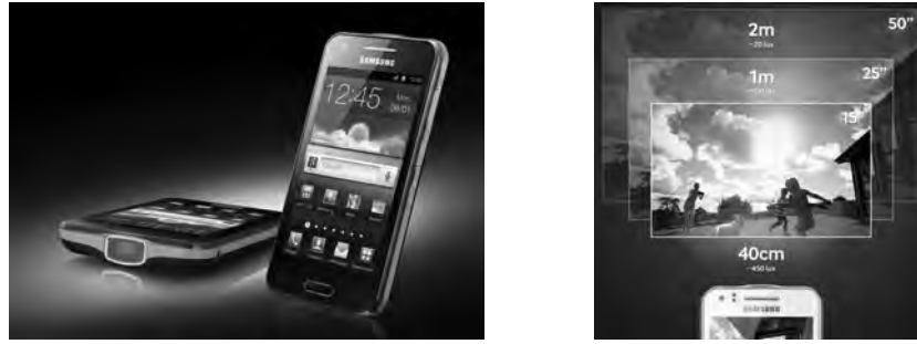
Figure 2.6: The Samsung Galaxy Beam projector-phone and its projection under different ambient lighting conditions (also see Subsection 2.4.1). It features a 15 Lumens projector, its successor the Galaxy Beam 2 (not shown) a 20 Lumens projector. Images courtesy of Samsung.
