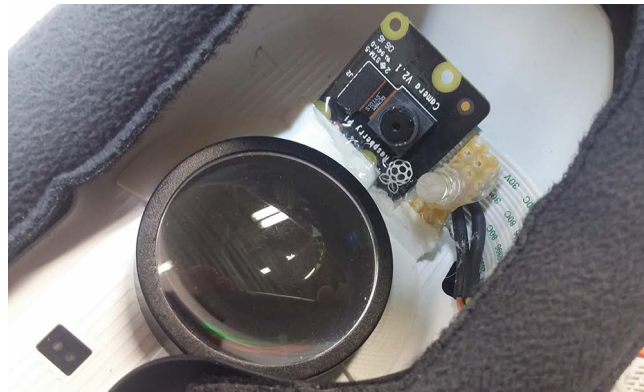
Figure 1: Hardware assembly inside the GearVR – the cables lead to a HDMI adapter board on the outside of the GearVR case.
