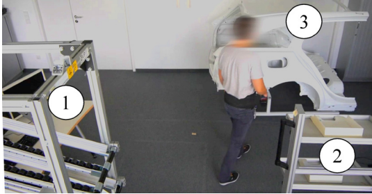
Fig. 5. Overview of the experimental setup: A participant had to successively pick up two screws at rack 1 and 2 and subsequently attach them to the work-piece (point 3).
