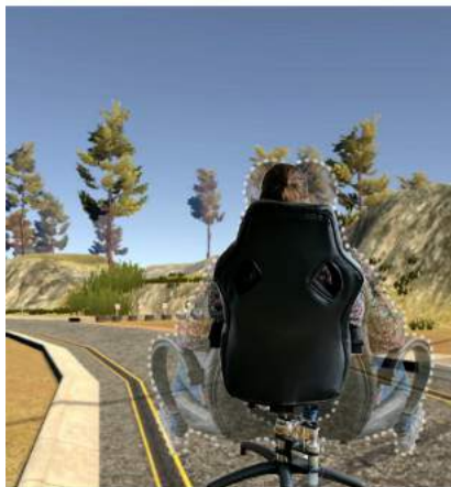
Figure 1. Forward motion approaches of VRSpinning to increase vection and reduce simulator sickness: wiggle movement to simulate steps or environmental events in VR (left middle), spin movement to simulate forward acceleration in VR by applying a short rotational impulse.
