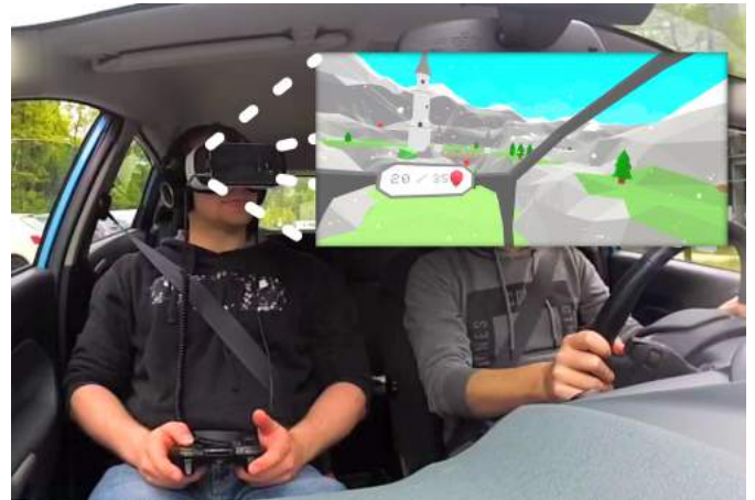
Figure 1. A player is sitting on the front passenger seat playing the game while the car is moving. Kinesthetic forces caused by the car match the movements in VR.
