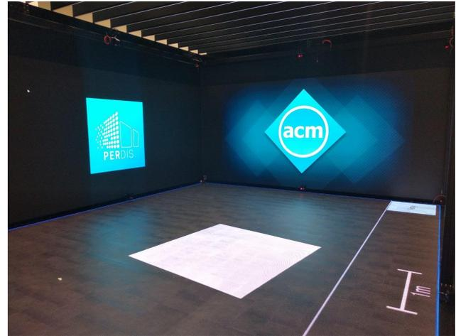
Figure 1: The apparatus consists of two L-shaped LED walls and a large scale LED floor setup.
