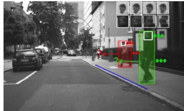
**Figure 2: Pedestrian path prediction of Kooij et al. [27]. Tracking bounding boxes of aware pedestrians are visualized green, head detection is visualized via a white box, and the curb with a blue line. Red indicates that the pedestrian is not aware of the oncoming vehicle.**
