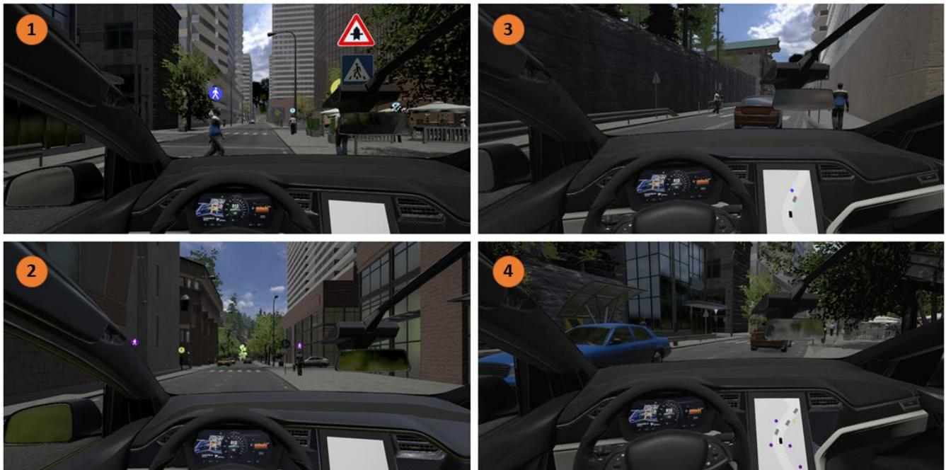
Figure 6: The interior of the simulated Tesla X alongside the visualizations: *AR three clarity states* (1), *AR two clarity states* (2), *tablet three clarity states* (3), *tablet two clarity states* (4).
