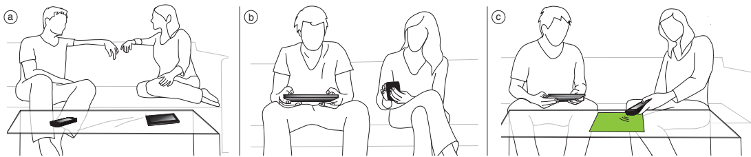
Figure 1. MobiSurf supports co-located decision making through integrating personal devices and a shared surface. a) Users discuss their goals. b) They can decide to work on the surface or their personal device. c) Information can be shared easily for discussion on the surface.
