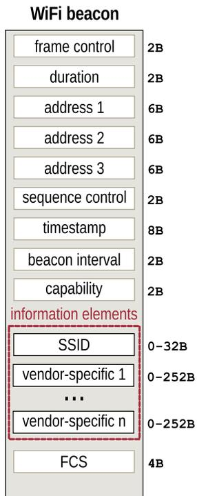
**Figure 1:** Frame format of WiFi beacons as defined in the IEEE 802.11 standard [4].
