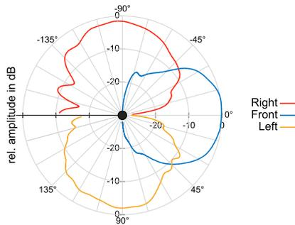
Figure 6: Radiation pattern of the dresser’s three build-in antennas, facing front (0°), right (-90°) and left (90°).
