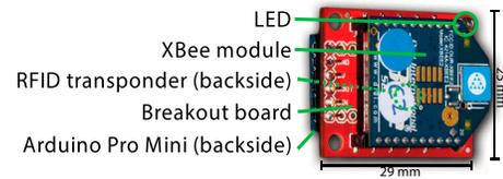
Figure 3: Stuff prototype based on Arduino.
