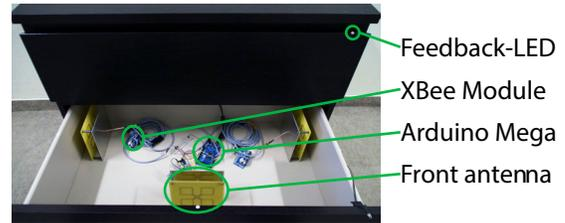
Figure 4: SmartFurniture prototype with three directed ZigBee antennas and Arduino controllers in the middle drawer.
