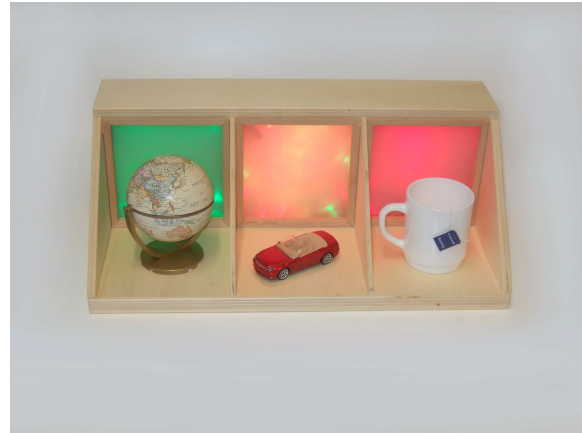
Figure 4: The ambient display subsystem of the Tangible Reminder, with an object in each tray, showing the different colors for different states.
