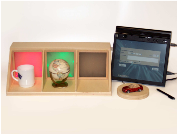
Figure 1: The Tangible Reminder system. The display subsystem on the left is showing different appointments, on the right hand a new appointment is being entered using the input subsystem.
