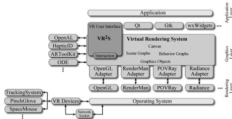
Figure 1: The system architecture of VRS ([2]) and its VR-based extension VR<sup>2</sup>S consisting of application, graphics and rendering layers.
