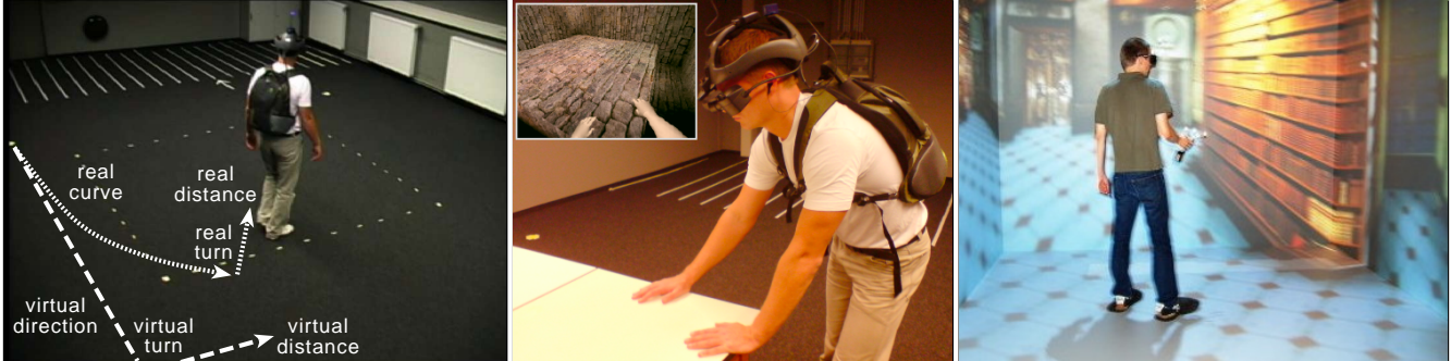
Figure 1: Concepts of the virtual holodeck: (left) a user walking through the tracked interaction space on a different path than the visually perceived counterpart, (middle) a user touching a real proxy object (the user's view is displayed as inset), and (right) a user in a six-wall CAVE in which a virtual room is displayed (by courtesy of CGV of TU Graz).
