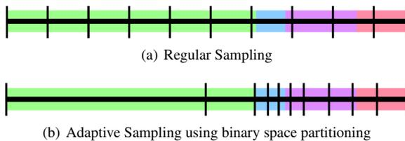
**Figure 5:** Comparison between equidistant and adaptive sampling. Vertical lines correspond to samples, different colors symbolize different paths. With regular sampling, green is oversampled while blue is not sampled at all. The adaptive sampling scheme samples all paths as evenly as possible.
