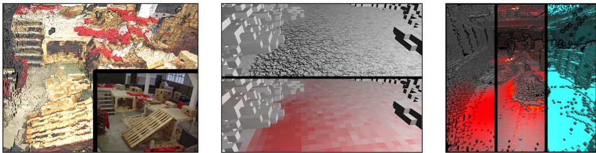
(a) Projective texturing applied to the Bremen Rescue Arena case with a handheld and manually positioned image (b) The occupancy for each voxel presented by bump mapping. The more occupancy a voxel has, the stronger the bump mapping effect is. (c) Attributes derived in the data pre-processing stage. From left: distance to the closest hazard, occupancy, and level of support
