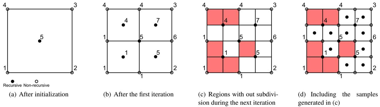
**Figure 4:** Adaptive sampling in two dimensions. Black dots are recursive samples, white dots are non-recursive, and numbers are identifiers for paths. There is a non-recursive sample for each corner and a recursive sample in the center (a). In each iteration, the central value is checked against each corner value and if they are different, new samples are created (b,c,d).
