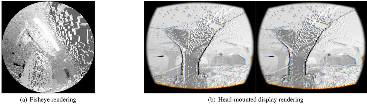
**Figure 7:** Two examples of immersive environments. Rendering the point cloud data in a portable dome environment (a) allows many people to analyze the data simultaneously, while head-mounted displays increase the immersion for a single user (b).
