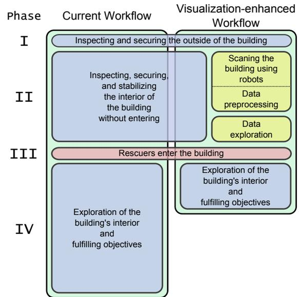
**Figure 2:** A schematic timeline overview of the currently employed workflow and our proposed system, showing events (red) and actions (blue) split up into four distinct phases. Utilizing additional actions (yellow) in parallel enables faster exploration and decreased overall time-to-rescue.
