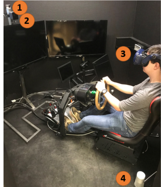
Figure 7: Study setup: camera (1), Vive base station (2), HTC Vive Pro (3) & speaker (4). While this participant holds on to the provided steering wheel, no manual driving was involved.
