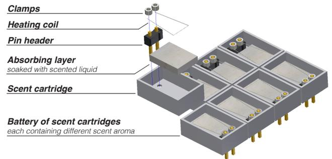
Figure 5. Overview of the scent cartridges with integrated heating units.
