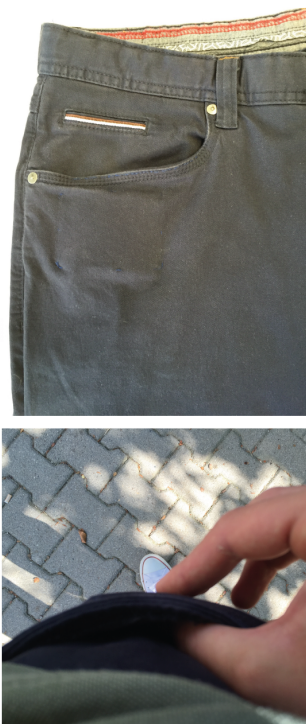
Figure 2: The PocketThumb interface is integrated into a common pair of trousers. The dual-sided touch sensor can be reached with the thumb from within the pocket and with the rest of the hand from the outside.
