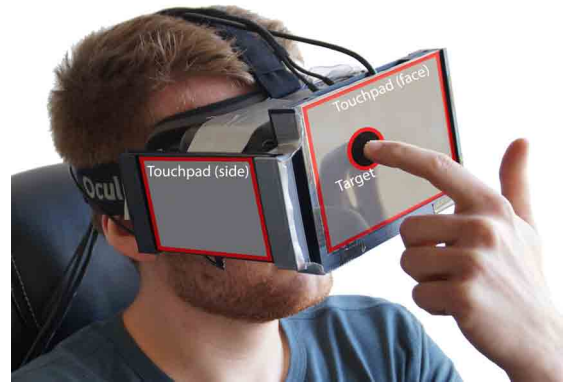
Figure 3. The FaceTouch prototype. A capacitive touchpad is embedded into a 3D-printed case and attached to the backside of an Oculus Rift DK2 via 5 small buttons that allow for pressure sensing on the touchpad. The side touchpad was only used in the second user study and does not have any buttons attached to it.
