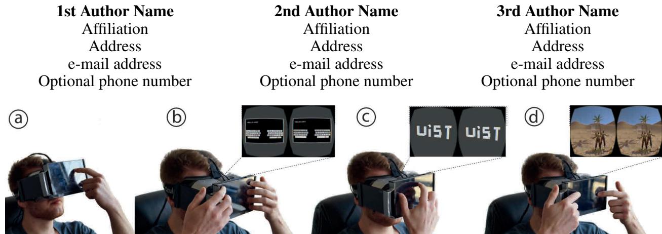
Figure 1. (a) A user interacting with FaceTouch , a multi-touch surface mounted on the back of a VR HMD. FaceTouch allows for precise interactions which can be used to implement applications such as text entry (b) or 3D modeling (c). Leveraging the sense of proprioception a user is able to blindly interact with control elements such as used in a gamepad to control a shooter game (d).
