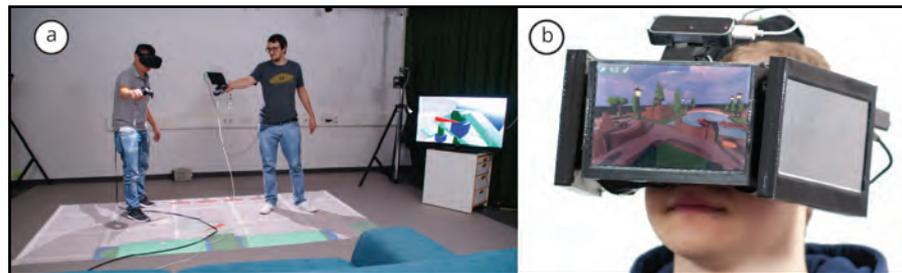
Figure 1.4: (a) Two users having an asymmetric interaction (HMD and non-HMD) with the ShareVR system using a tracked display and a floor projection to visualize the virtual world for the non-HMD user [Core5]. (b) A user wearing the FaceDisplay prototype, a modified VR HMD consisting of three touch sensitive displays and a depth camera attached to its back [Core6].
