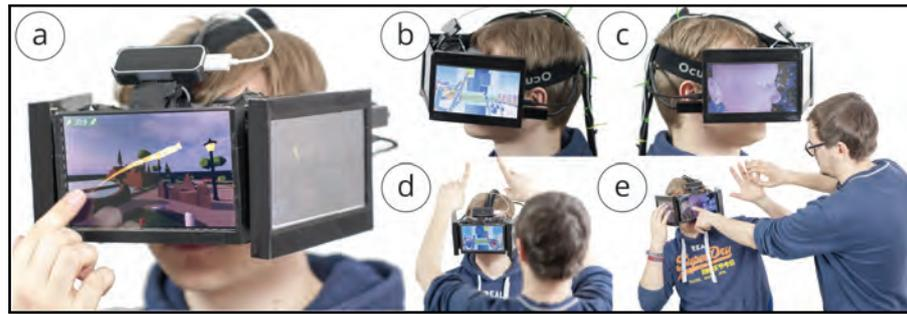
**Figure 3.8:** The FaceDisplay prototype, a modified VR HMD consisting of three touch sensitive displays and a depth camera attached to its back (a-c). This allows people in the surrounding to perceive the virtual world through the displays and interact with the HMD user either through touch (e) or gestures (d) [Core6].
