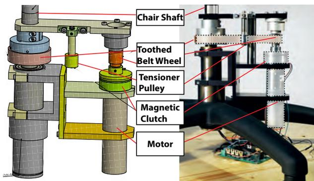
Figure 3. On the left, the 3D model of the chair construction and on the right the actual implementation showing the attachment to the chair
