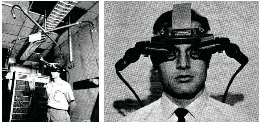
**Figure 1.1:** (left) The *Sword of Damocles* system mounted on the ceiling and consisting of two (right) miniature cathode ray tubes [228]
