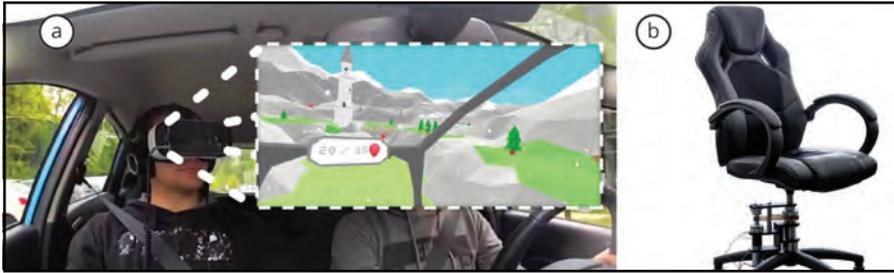
**Figure 1.5:** (a) A user sitting in the front passenger seat and interacting with the CarVR system which maps the physical rotation of the car into the virtual environment [Core4]. (b) The physical prototype of the SwiVRChair system, consisting of a modified office chair with a motor and a clutch, enabling to nudge a users orientation inside the virtual environment [Core3]
