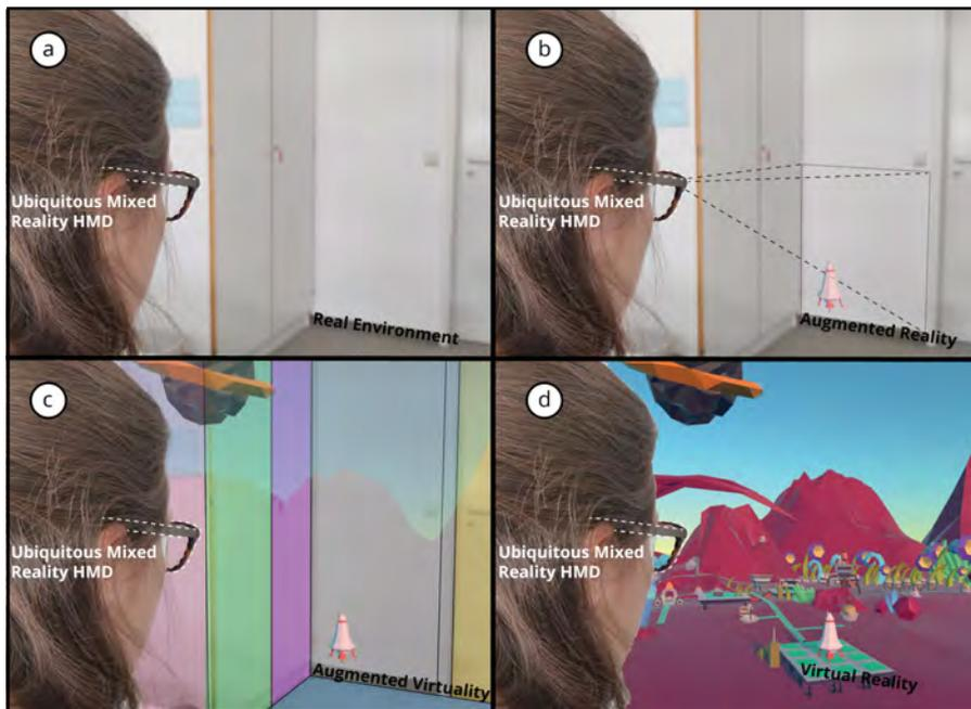
**Figure 2.3:** An envisioned ubiquitous mixed reality HMD capable of effortlessly transition along the reality-virtuality continuum and able to extend the (a) real environment using (b) augmented reality, (c) augmented virtuality and (d) virtual reality.
