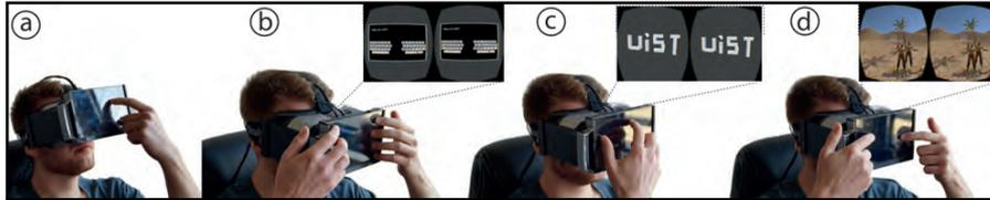
Figure 3.3: (a) A user interacting with FaceTouch, a multi-touch surface mounted on the back of a VR HMD. FaceTouch allows for precise interactions which can be used to implement applications such as text entry (b) or 3D modeling (c). Leveraging the sense of proprioception a user is able to blindly interact with control elements such as used in a gamepad to control a shooter game (d) [Core1].
