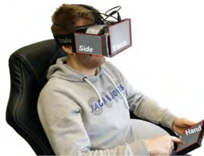
Figure 8. Placement of the touchpads during the positioning user study
