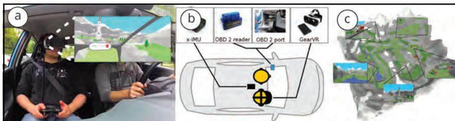
Figure 3.5: (a) A user interacting with CarVR on the front passenger seat playing a game while the car is moving. (b) Schematic overview of the technical setup used to implement CarVR. (c) The modeled scene used for the study. The five small images show the view from the ego perspective but without the cockpit [Core4].
