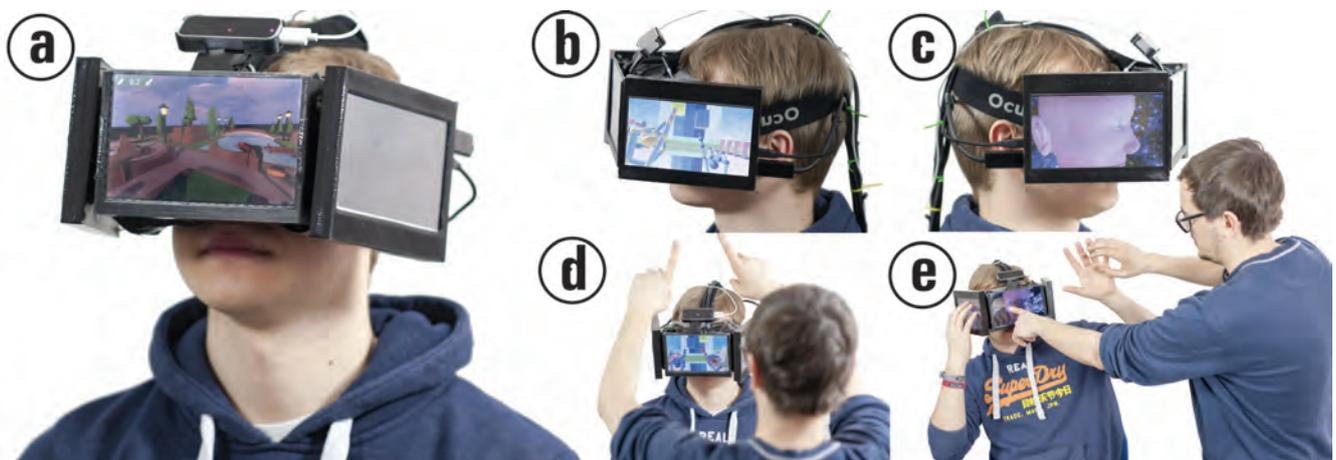
**Figure 1.** FaceDisplay is a modified VR HMD consisting of three touch sensitive displays and a depth camera attached to its back (a-c). This allows people in the surrounding to perceive the virtual world through the displays and interact with the HMD user either through touch (e) or gestures (d).
