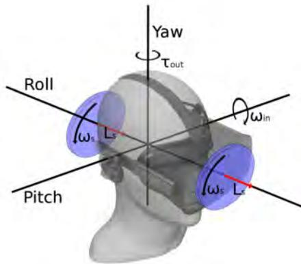
Figure 4. When disks are spun with angular velocity  $\omega_s$  and the head is rotated around an input axis at angular velocity  $\omega_{in}$ , the gyroscopic output torque  $\tau_{out}$  around the yaw axis is experienced by the user.
