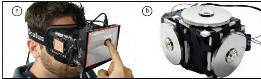
Figure 1.3: (a) A user interacting with FaceTouch, a multi-touch surface mounted on the back of a VR HMD [Core1]. (b) A first prototype implementation of GyroVR consisting of attached flywheels on each rotational axis of an Oculus Rift DK2 [Core2].
