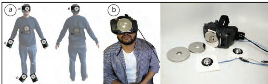
**Figure 3.4:** (a) The different mounting positions on the human body which were explored with the mobile implementation of GyroVR. (b) A user wearing a VR HMD with GyroVR attached and a prototype implementation of GyroVR attaching flywheels on the front of an Oculus Rift DK2 [Core2].
