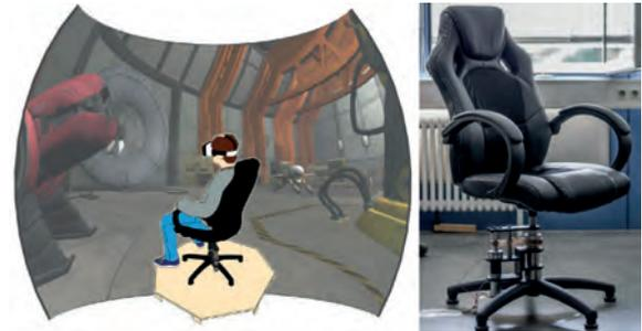
Figure 1. Left: A participant being rotated inside a virtual scene sitting on the *SwiVRChair*. Right: The physical prototype of the *SwiVRChair*
