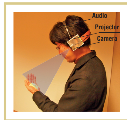
Figure 3. The Brainy Hand system. It envisions the camera-projector system as an earpiece for interactive projection onto the user's hand. (Source: Emi Tamaki and her colleagues; used with permission.)
