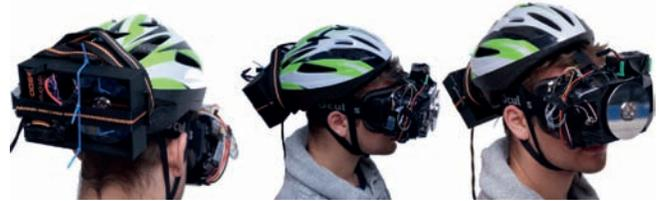
**Figure 8.** The study apparatus of GyroVR consisting of a Oculus Rift DK2 with GyroVR attached and a bicycle helmet having a mobile GyroVR prototype attached to the back.
