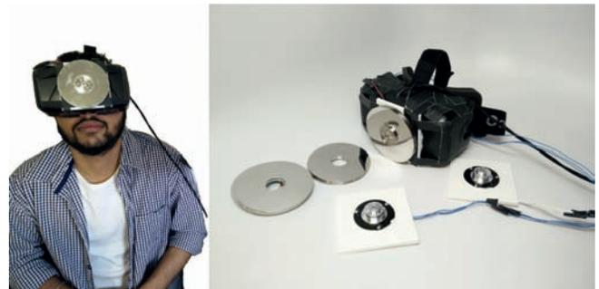
Figure 1. Left: A user wearing a VR HMD with GyroVR attached. Right: A prototype implementation of GyroVR attaching flywheels on the front of an Oculus Rift DK2.
