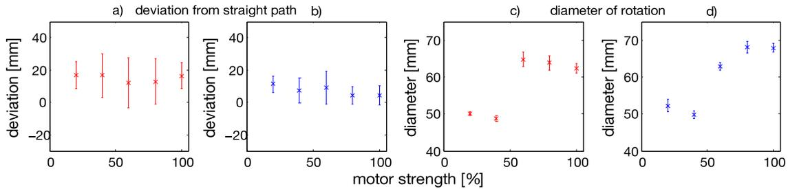
**Figure 4. Results from two different experiments. The two leftmost graphs show the absolute deviation from a straight path for 5 different motor settings and 2 different lengths of bristles (red short, blue long). The two rightmost graphs show the diameter for circular motion (just one motor active).**
