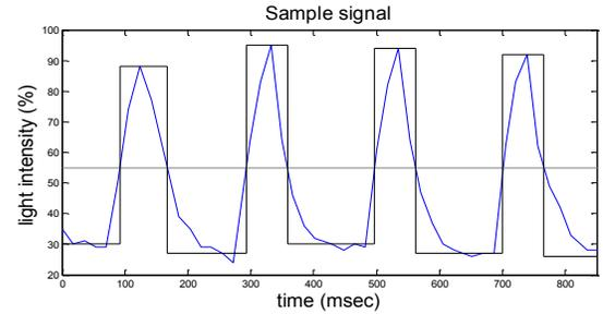
Figure 3. An illustration of the light signal which is sent by the tangibles LEDs.
