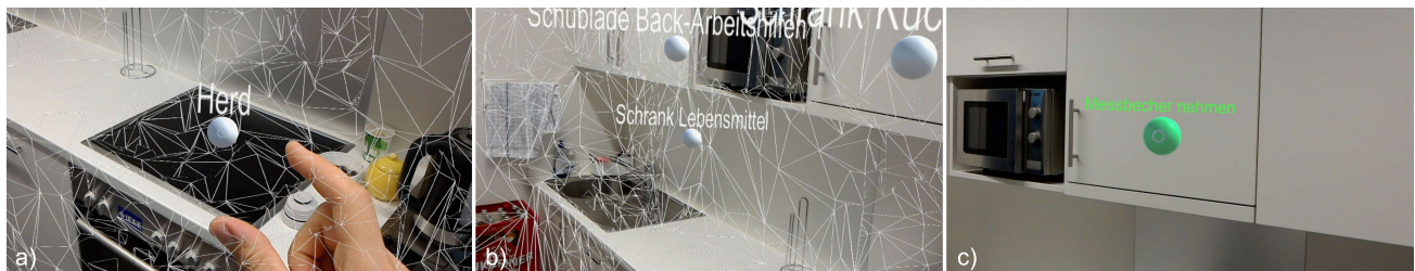
Figure 1. a) Using pinch gestures, caregivers can place key-areas for instructions on the room model generated by the HoloLens. (b) After each key-area has been defined, instructions are displayed at their corresponding position (c).
