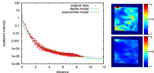
Figure 1: *Left*: Comparison of the fitting accuracy for measured input data. Note how close the exponential model approximates the data, especially in the region around the point of incidence where the dipole model starts off too high and falls too steeply. *Right*: Color coded reconstruction error for a planar sample of marble. The top image shows the error for the isotropic model, the bottom image for an anisotropic model with  $m = 8$ .
