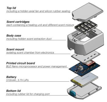
Figure 2. Overview of the assembly of the inScent prototype.
