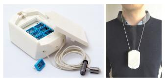
Figure 3. Left: The *inScent* prototype with opened top lid. Up to 8 scent cartridges can be plugged in. Each cartridges contains highly viscous scented liquid soaked into glass fiber to deter leaking. Right: Normally, scent emission is not visible to the eye. For this photo, we highly increased the amount of glycerol to make the scent emission visible as smoke.
