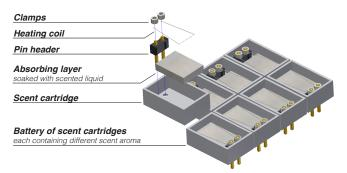
Figure 5. Overview of the scent cardriges with integrated heating units.
