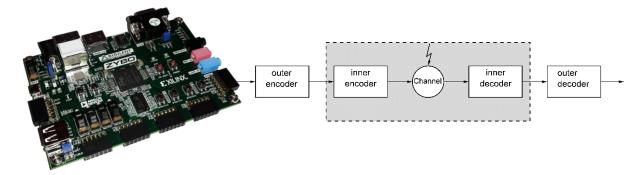
The goal of this thesis will be the implementation of concatenated codes using Reed-Solomon codes as their components on a Xilinx FPGA. The hardware has to be optimized for runtime and area efficiency. With an existing test framework the functionality with real PUF responses has to be evaluated and compared to existing implementations of other error correction techniques.
