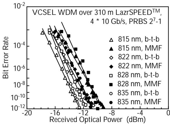
Fig. 4. Bit error rates for all four channels versus optical power at the receiver for 10 Gb/s back-to-back (b-t-b) operation and transmission over 310 m of 50  $\mu\text{m}$  core diameter MMF cable.
