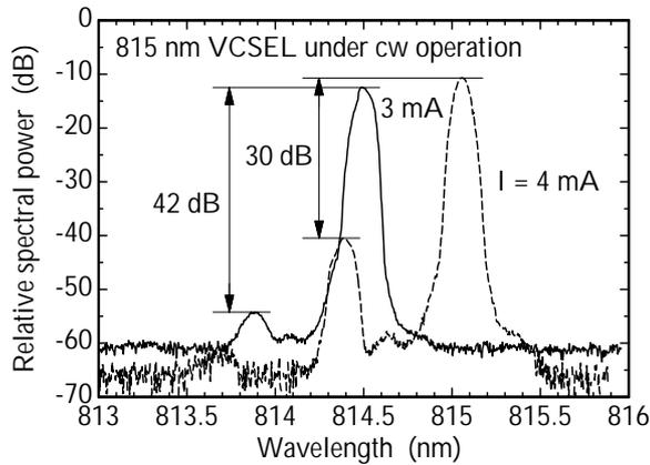
Fig. 2. Optical spectra of the 815 nm device for 3 and 4 mA driving currents.
