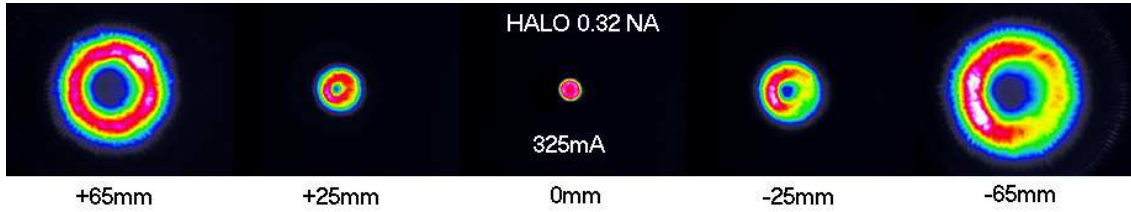
Fig. 2: Captured images of a 80\ \mu\text{m} active diameter VCSEL beam at different positions from the beam waist.
