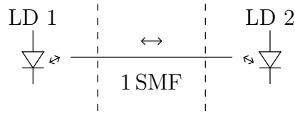
Fig. 2: Schematic of our bidirectional approach incorporating two identical FP lasers.
