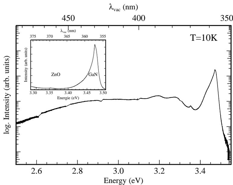
**Fig. 4:** Low temperature photoluminescence of GaN nanotubes.
