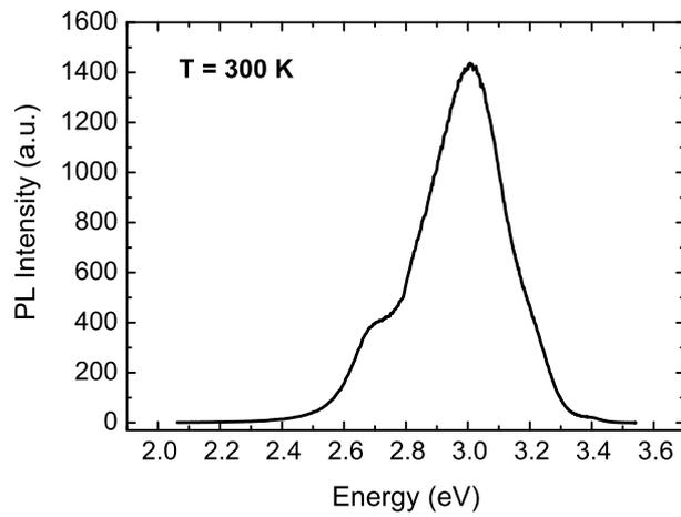
**Fig. 6:** Room temperature photoluminescence of GaInN GaN coaxial nanotube structures.
