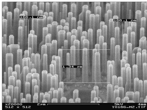
Fig. 1: ZnO nanorods grown on a-plane sapphire.
