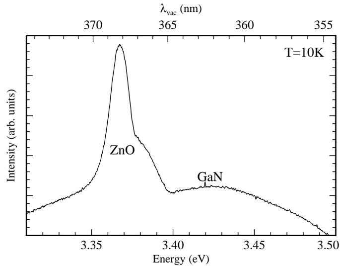
**Fig. 2:** Low temperature photoluminescence of GaN-ZnO coaxial nanorods.
