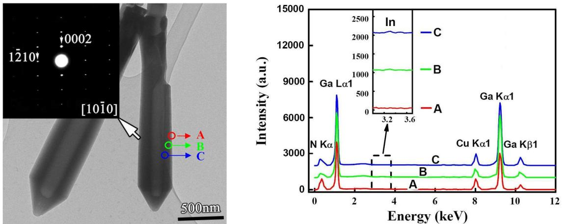
**Fig. 7:** TEM analysis (left) and related EDX analysis of a GaInN GaN coaxial nanotube structure. The inset (left) shows an electron diffraction signal taken along the  $[10\bar{1}0]$  zone axis of the nanocolumn confirming its crystalline character.
