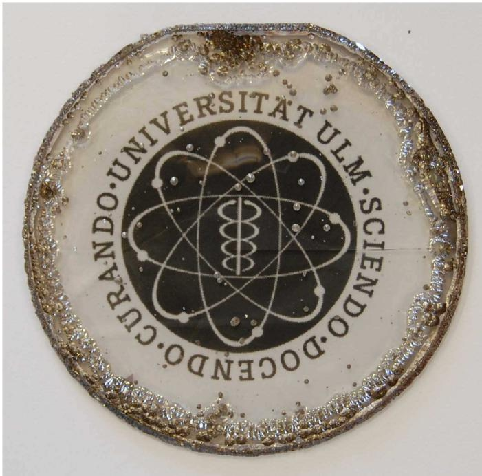
**Fig. 4:** Photograph of a full 2" GaN wafer self-separated during cool-down by growth on the hexagonally shaped mask with a period of 30  $\mu\text{m}$ . The thickness of the wafer is about 1.5 mm.
