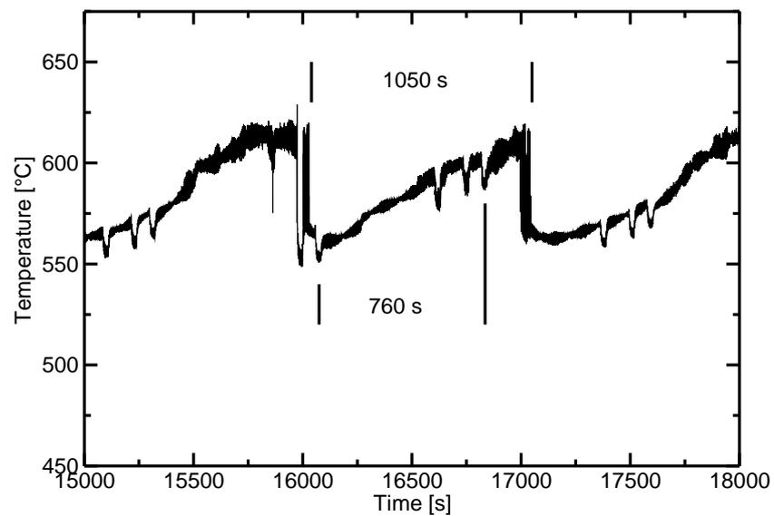
**Fig. 8:** Detailed temperature plot during growth of sample B. The oscillation period of  $\approx 1050$  s is not equal to the growth time of one Bragg mirror period (760 s).
