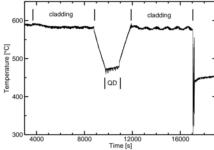
**Fig. 5:** Temperature profile determined with band-edge absorption spectroscopy of sample A. The oscillations during growth of the second cladding layer are no real fluctuations of the sample temperature but are caused by the measurement method.
