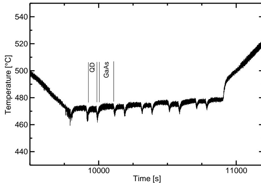
**Fig. 6:** Detailed time-dependent temperature during growth of the quantum dot active region of sample A. The temperature dips indicate closure of all shutters for 10 seconds, separating quantum dot and barrier material growth.
