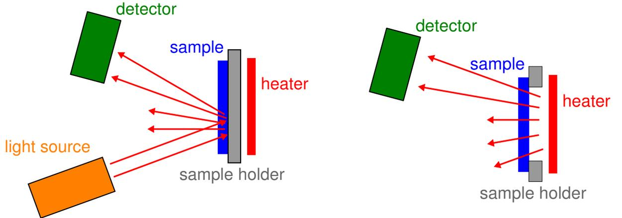
**Fig. 1:** Schematic drawing of the reflection mode (left) and the transmission mode (right) of band-edge absorption spectroscopy. The reflection mode requires an external light source and one additional viewport in the growth chamber.
