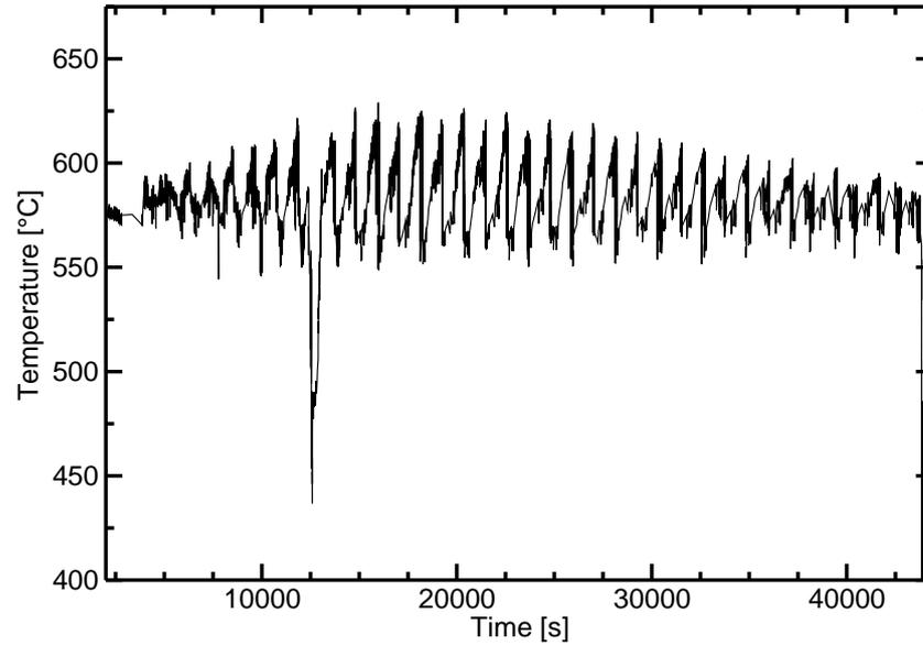
**Fig. 7:** Temperature profile determined with band-edge absorption spectroscopy of sample B. The spectral influence of the Bragg mirror layers on the detected signal lead to strong spurious temperature fluctuations.
