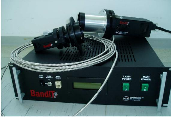
**Fig. 3:** Hardware of the BandiT band-edge absorption spectroscopy system, consisting of a controller with spectrometer, a fiber-coupled detector head and a halogen lamp.
