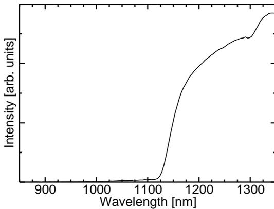
**Fig. 2:** Transmission spectrum of light passing through an undoped GaAs substrate at a temperature of 582 °C (verified by RHEED transition).
