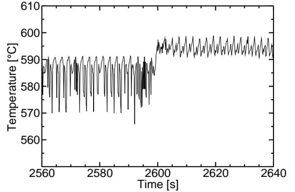
**Fig. 4:** Spurious temperature oscillations caused by the rotation of the substrate. At 2600 s, the Ga shutter was opened, which results in a rise of the sample temperature.
