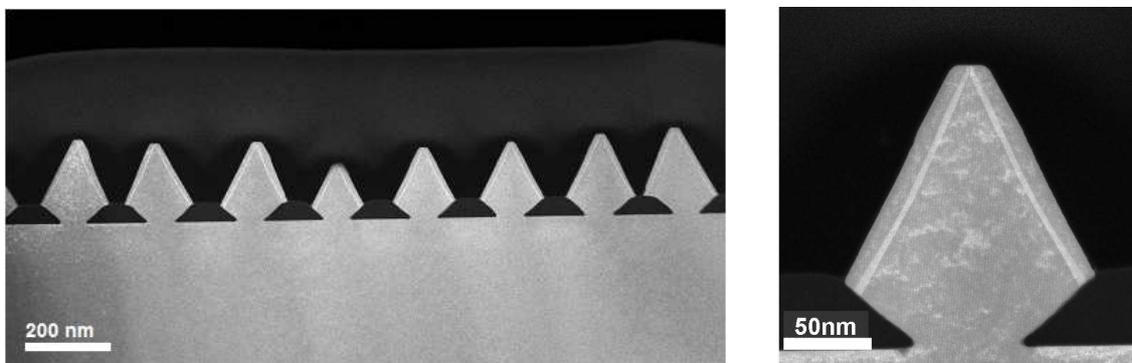
**Fig. 9:** TEM cross-section images of GaN stripes with semipolar InGaIn/GaN quantum wells on the sidefacets.
