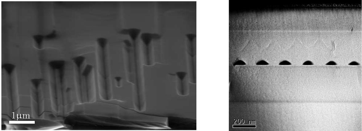
**Fig. 10:** Comparison of the embedding for different orientations. The SEM picture on the left (topview) shows a sample with stripes oriented along  $a$ -direction with  $\{10\bar{1}1\}$  facets being incompletely planarized whereas the TEM picture on the right (cross-section) shows the immaculate embedding of a structure with  $\{11\bar{2}\}$  side facets.
