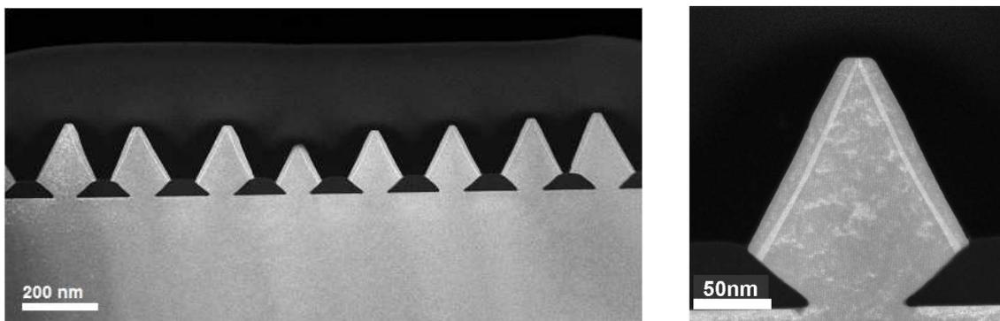
**Fig. 9:** TEM cross-section images of GaN stripes with semipolar InGaN/GaN quantum wells on the sidefacets.
