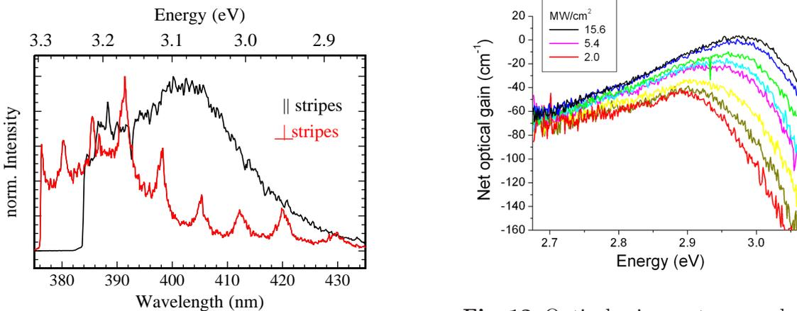
**Fig. 11:** PL spectra recorded for light emission  $\parallel$  and  $\perp$  to the stripes.
