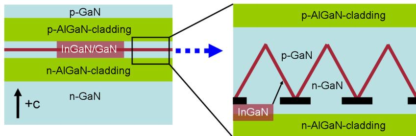
**Fig. 8:** Shrinking the size of the 3D structures allows the integration of semipolar quantum wells inside a conventional laser diode grown in polar direction.
