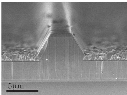
**Fig. 7:** SEM cross-section of stripes parallel  $a$  with  $\{10\bar{1}1\}$  side facets. The GaN ridge on top of a truncated AlGaN stripe is clearly visible. Parasitic nucleation on the mask led to polycrystalline growth.
