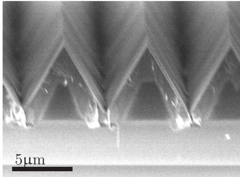
**Fig. 6:** SEM cross-section of stripes parallel  $a$  with  $\{10\bar{1}1\}$  facets. The GaN core is overgrown by a thick AlGaN layer.
