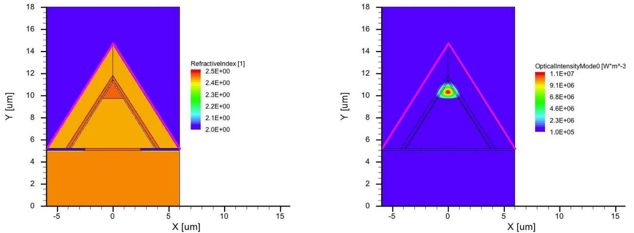
**Fig. 3:** Concept and simulation of the optical modes for concept SM1. A triangular GaN stripe is grown on top of a truncated AlGaIn stripe and consequently enclosed by an upper AlGaIn cladding.
