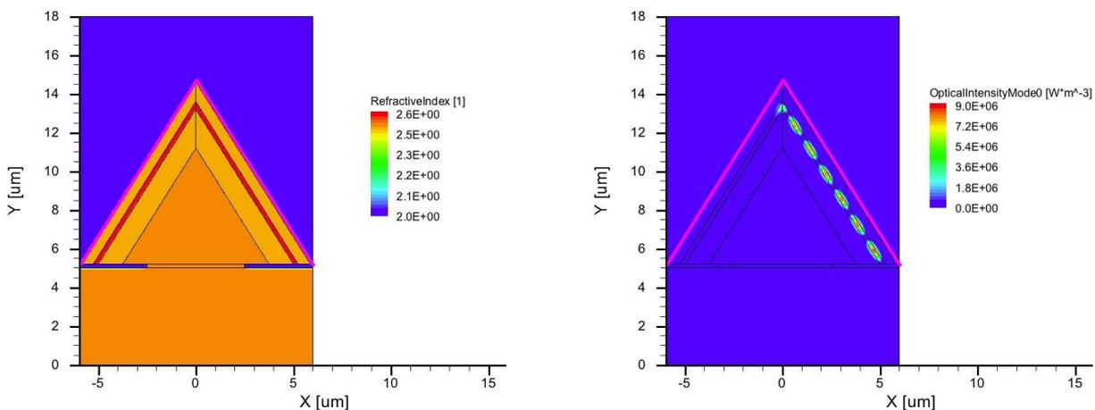
**Fig. 2:** Concept and simulation of the optical modes for a concept of AlGaIn/GaN/AlGaIn layers deposited on the side facets of a GaN stripe with triangular cross-section.
