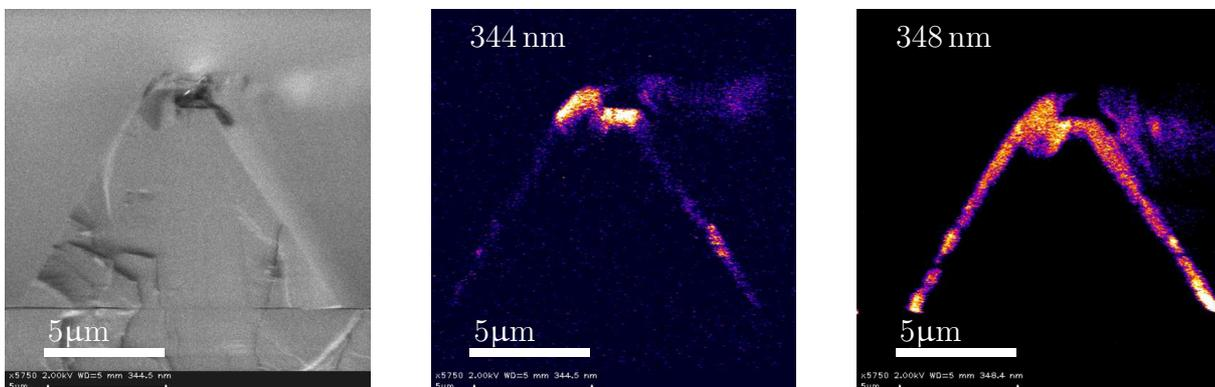
**Fig. 5:** SEM cross-section and monochromatic CL mappings at 8K of stripe parallel to  $m$  with  $\{11\bar{2}2\}$  facets. The thin cladding layer of AlGaN is clearly visible. The top of the stripe exhibits luminescence at a higher energy as result of a higher aluminum incorporation.
