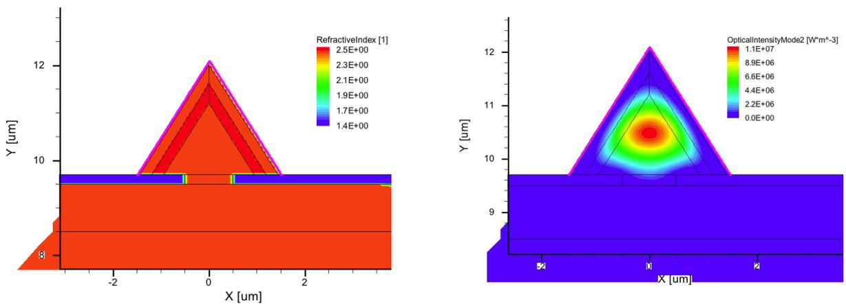
**Fig. 4:** Concept and Simulation of the optical modes for concept SM2. A planar AlGaIn layer is included in the template as the bottom cladding. The waveguide core is directly grown on the template and only one 3D growth step for AlGaIn is needed.
