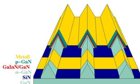
**Fig. 1:** Realization of a LED with semipolar quantum wells on the sidefacets of GaN stripes with triangular cross-section.
