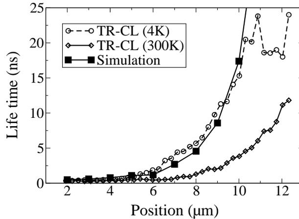
**Fig. 4:** Carrier life time along inverse pyramid facet. Position 0 corresponds to the inner tip.
