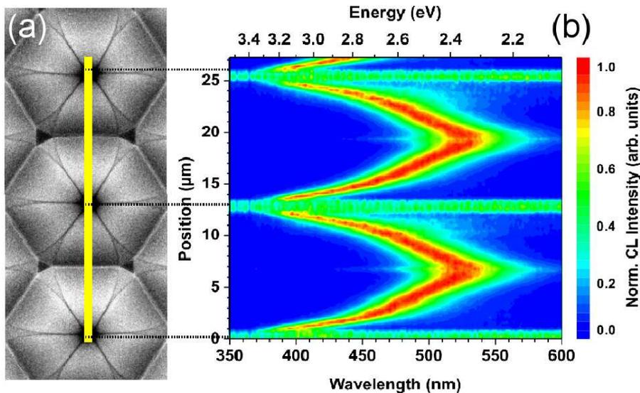
**Fig. 1:** SEM top view of inverse pyramid structure with  $\{11\bar{2}2\}$  facets and a period length of  $13\ \mu\text{m}$  (a) and respective CL wavelength linescan (b). The data was acquired by S. Metzner, Otto-von-Guericke-Universität Magdeburg.
