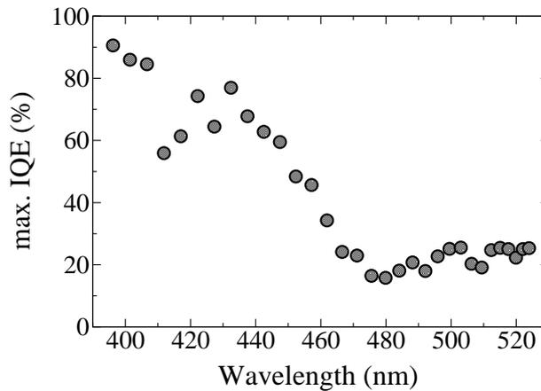
**Fig. 7:** Max. IQE vs wavelength determined using Equ. 3 and the carrier life times from Fig. 4.
