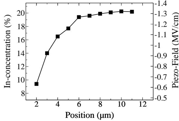
**Fig. 5:** In-composition along inverse pyramid facet. Position 0 corresponds to the inner tip.
