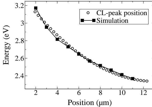
**Fig. 3:** QW transition energy along inverse pyramid facet. Position 0 corresponds to the inner tip.
