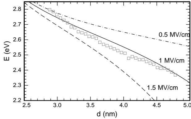
**Fig. 6:** CL emission energy along upper half of inverse pyramid in correlation with determined QW thickness (squares) (section 4). Shift of emission energy for different field strengths using the analytic model of Bulashevich et al. [17]. Curves are normalized.
