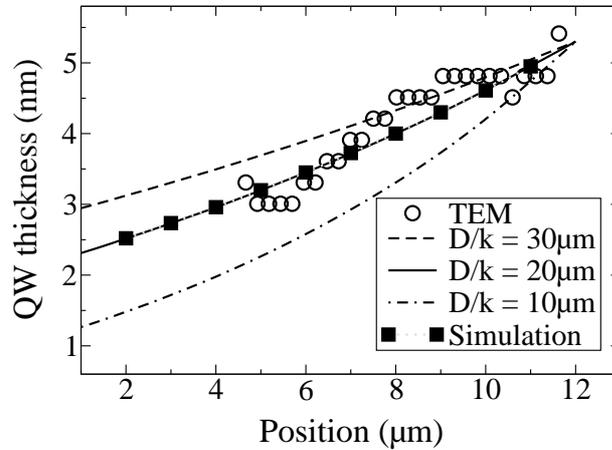
**Fig. 2:** QW thickness along inverse pyramid facet. Position 0 corresponds to the inner tip.
