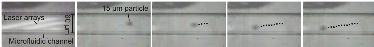
Fig. 7: Deflection experiment with a 15\ \mu\text{m} polystyrene particle inside a microfluidic channel. The particle is stepwise redirected by the VCSELs in the array.
