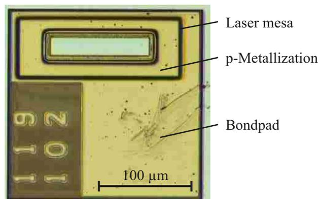
**Fig. 1:** Top view of a fully processed rectangular-shaped VCSEL. The oxide aperture is around  $100 \times 14 \mu\text{m}^2$ . The rectangular laser mesa as well as the bondpad are clearly visible.
