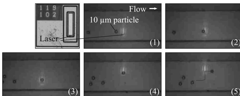
**Fig. 4:** Optical manipulation of a single 10 μm polystyrene particle under flow inside a 75 μm microfluidic channel. In this experiment, the flow track of the particle is manipulated.
