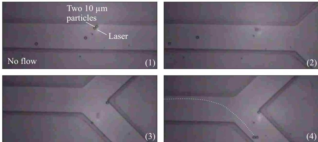
**Fig. 5:** Simultaneous optical trapping of two 10  $\mu\text{m}$  polystyrene particles without flow inside a 60  $\mu\text{m}$  microfluidic channel. In this experiment, particle sorting is achieved by placing them in the desired branch of the Y-junction.
