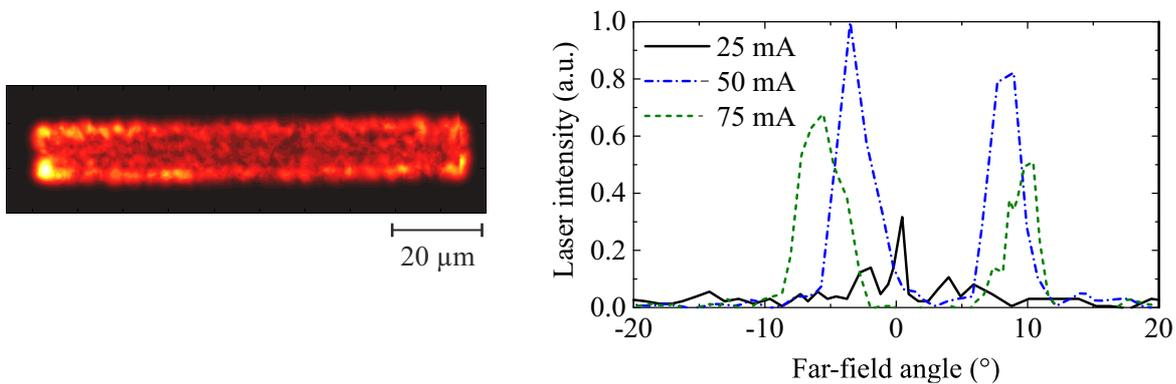
**Fig. 3:** Near-field (left) and long-axis far-field (right) of the rectangular VCSEL used for optical manipulation. The near-field was measured at 85 mA and the far-field at three different currents between threshold and roll-over.
