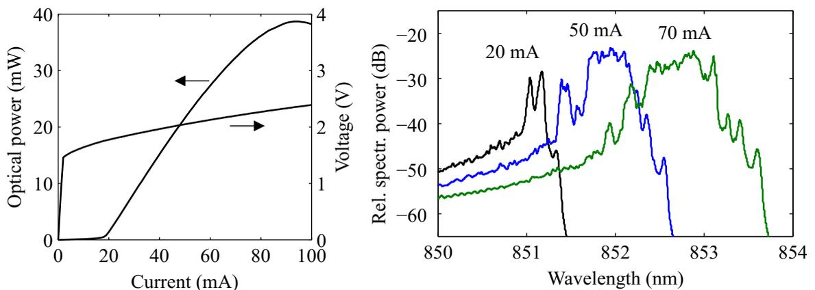
**Fig. 2:** Light–current–voltage characteristics (left) and optical spectra (right) of the rectangular VCSEL used for optical manipulation. The spectra are measured at three different currents between threshold and roll-over.
