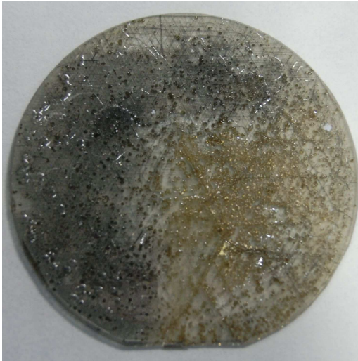
Fig. 1: Free-standing Fe-doped GaN sample on a template with 30 \mu\text{m} mask period. Fe content according to SIMS: 2 \cdot 10^{18} \text{ cm}^{-3} .
