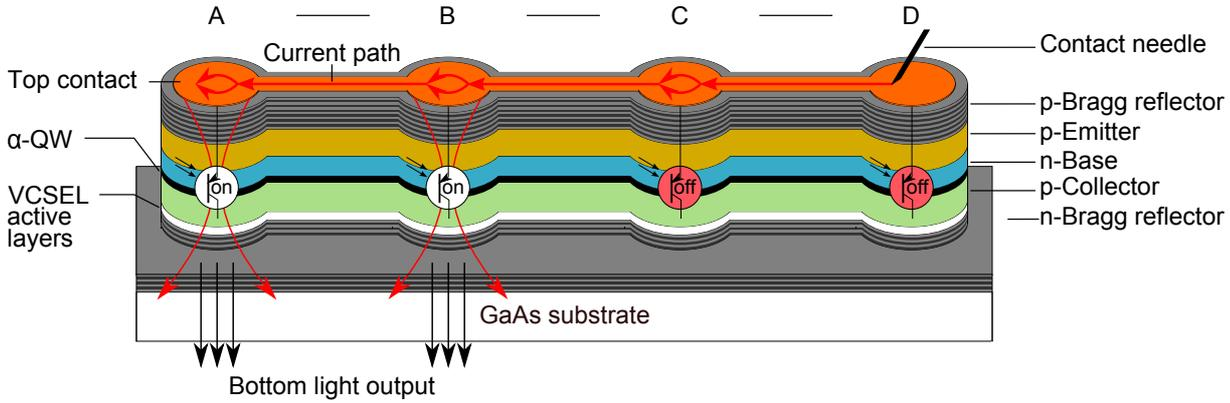
**Fig. 1:** Layout and operation principle of the four parallel-driven bottom-emitting VCSELs with integrated phototransistor layers for optically controlled current confinement. Initially, the phototransistor with the lowest voltage drop during dark-current operation begins to open and becomes conductive. The resulting spontaneous photons reach the neighboring mesas through the thin ridges and switch them on successively.
