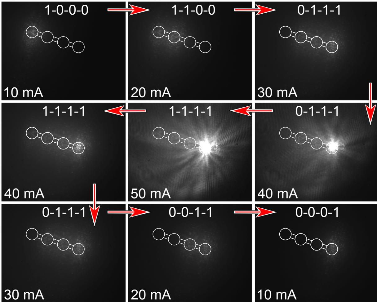
**Fig. 4:** Camera images of the bottom side of the PT-VCSEL arrangement at different currents during turn-on and -off. The four parallel-driven mesas are highlighted in white. “0” and “1” represent the off-/on-state of the PT in each mesa. The needle contacts the right mesa (position D in Fig. 1).
