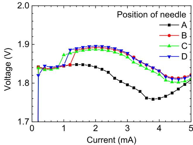
**Fig. 3:** Current-voltage measurements of the leakage current in the dark-current region for all contact positions of Fig. 1. For each trace, the pump current is reduced from 50 mA to zero to ensure the needle-contacted PT turns off last. Only the range from 0 to 5 mA is shown here. The voltage drop of the left mesa (position A) is less than of the others. Hence, due to the highest initial photon density, this PT always begins to turn on first.
