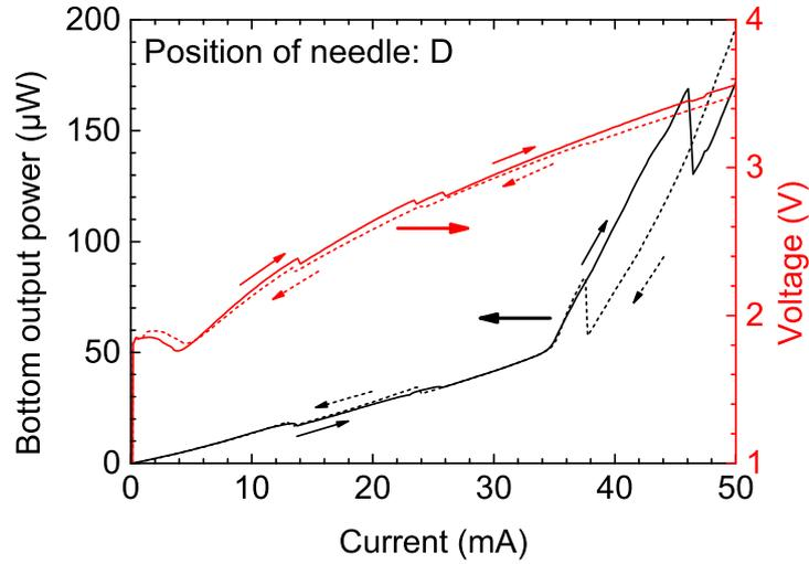
**Fig. 2:** Measured continuous-wave operation curves of the four parallel-driven PT-VCSELs. Each kink indicates a turn-on/-off point of a PT. The turn-off order of the PTs is different from that during turn-on, hence hysteresis loops exist.
