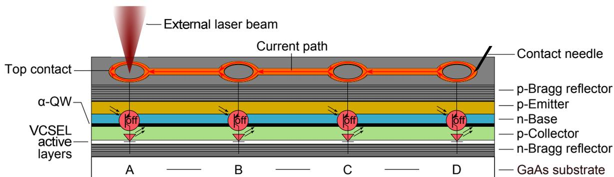
**Fig. 2:** Schematic layout of parallel-driven PT-VCSELs which are defined by four interconnected surface metal contact rings. The external laser beam is focused at position A and introduces additional photons in the resonator.
