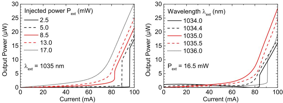
**Fig. 5:** Measured LI curves of a bottom-emitting PT-VCSEL with a contact ring diameter of 230  $\mu\text{m}$  while varying the injected optical power (left) and the wavelength of the external laser source (right).
