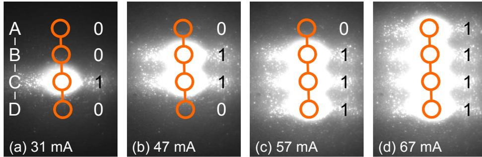
**Fig. 3:** CCD camera images of the bottom side of spontaneously emitting PT-VCSELs according to Fig. 2. The top metal contact structure is highlighted in orange. “0” and “1” represent the off-/on-state of each PT, respectively, and the turn-on currents where the individual PTs become locally conductive are displayed at the bottom. As in Fig. 2 the needle contacts an outer ring at position D. The turn-on order is C–B–D–A.
