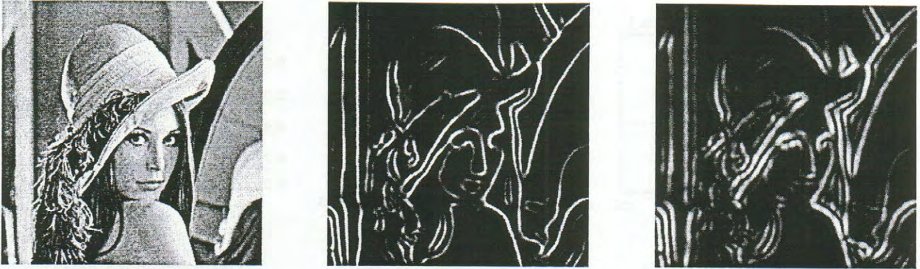
Figure 7: Processing a real camera image (left). Pooled activity of all orientation fields generated by the non-linear circuit (center) vs. the linear model (right). Note, that no further post-processing, such as local non-maximum suppression, has been applied to the data.
