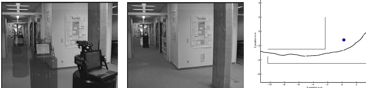
Figure 6: Experiment showing successful navigation down the middle of a hallway. Left : superposition of three snapshots from the beginning of the sequence. Middle : snapshot towards end of sequence with robot at end of hallway. Right : top view of the robot trajectory (from odometry) in the hallway (sketch based on laser scan).
