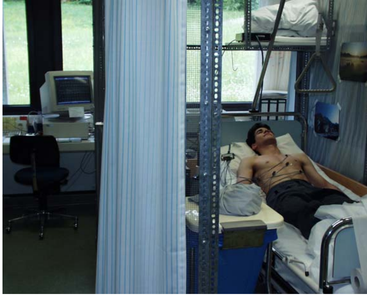
Figure 5. Picture of the high resolution ECG recording facilities. The subject is lying inside the Faraday cage.
