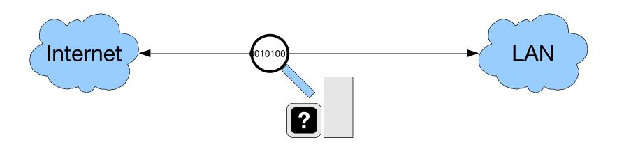
**Packet Filtering Router**
