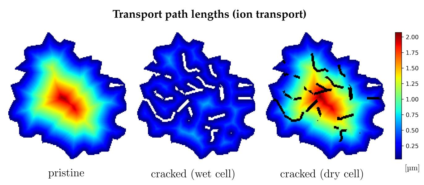
Realizations of the stochastic 3D for cracked particles can be utilized to investigate the change of path lengths before (left) and after cracking. The change of path lengths for ion transport depends on the kind of battery. In wet cell batteries, cracks are flooded with electrolyte, resulting in shorter paths (middle). Conversely, in dry cell batteries, cracks typically serve as obstacles, leading to an increase in path lengths (right).
