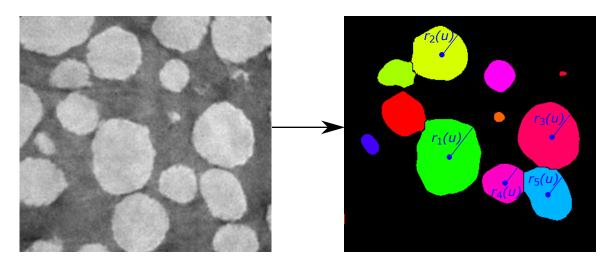
Nano-CT data of NMC particles is segmented [4]. Particles are represented by radius functions  $r_1, \ldots, r_n$ :
