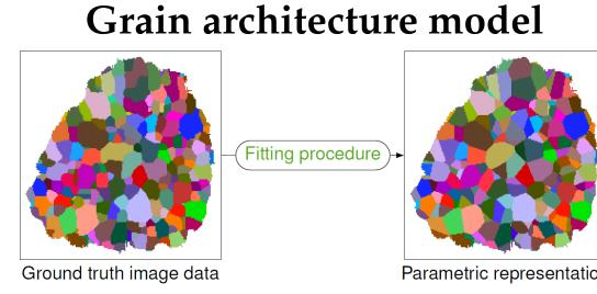
Parametric representation  $\{(y_i, r_i)\}_{i=1}^n \subset \mathbb{R}^4$ of segmented 3D EBSD data by Laguerre tessellation is determined [3]. The *i*-th cell of the tessellation is given by
