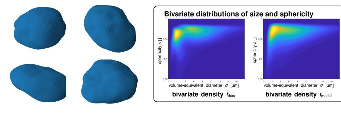
Isotropic Gaussian fields R (on the sphere) can be used to model radius functions [4]. The parameters of a mixture of Gaussian fields are fitted to  $r_1, \ldots, r_n$ .
