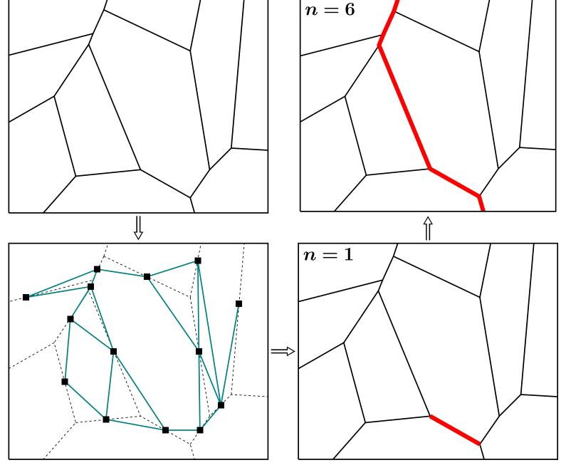
The grain architecture is represented as adjacency graph of grain boundaries (facets). A crack is modeled by choosing an initial facet followed by iteratively adding neighboring facets, based on their alignment w.r.t. the priorly chosen facet path [8]. Finally, the chosen facets are dilated to model the crack.
