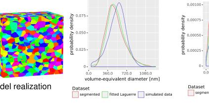
The grain architecture model is derived by fitting a stochastic model to the marked point pattern  $\{(y_i, r_i)\}_{i=1}^{n}$  [4].
