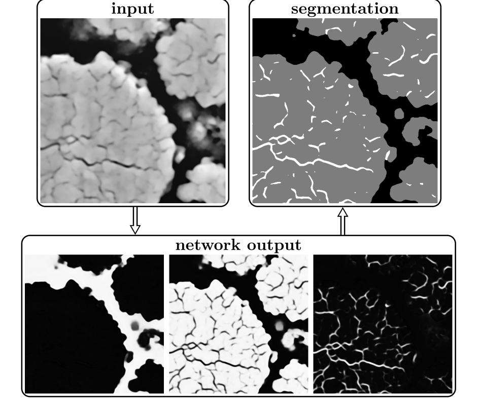
A U-net [6] is trained to segment (super-resolved [7]) SEM images into background, cracks and solid phase.
