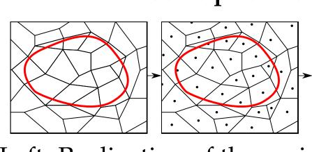
Left: Realization of the grain architecture and outer shell. Center: Centers of mass for each grain. Right: Deletion of grains whose centers are not in the outer shell.
