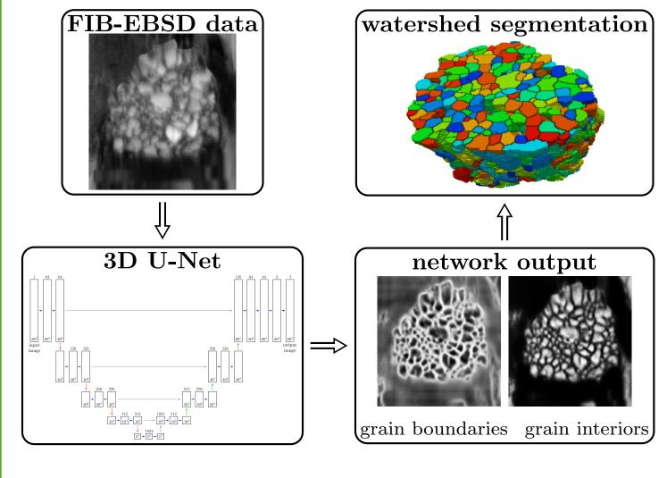
A 3D U-Net [1] was trained to enhance grain boundaries in FIB-EBSD data. Then, a grain-wise segmentation is computed, utilizing a marker-based watershed algorithm [2].
