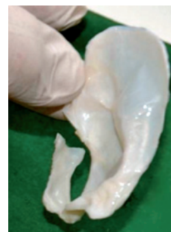
Bacterial nanocellulose in the shape of a human auricle
