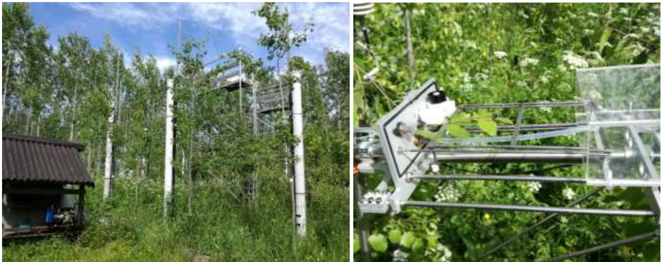
Figure 3: FAHM experimental site in Järvselja, Estonia. On the left: the air humidity is manipulated in young deciduous (silver birch and hybrid aspen) forest stands through misting water under high pressure. Such technology enables to increase air relative humidity up to 18% unit above ambient level. Photo credit: Liisi Tõnisson.
